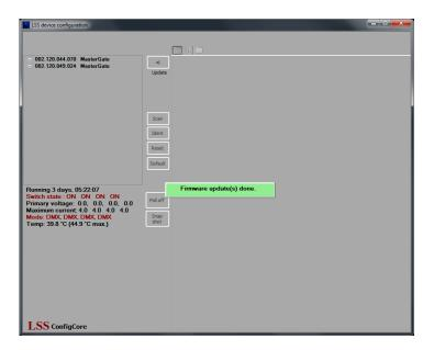
At the end of the update, the control unit of the *MasterPort 2 PSU* is reset. After reset in ConfigCore still the old Art-Net device name and the old version number is displayed. That is normal until loading the default settings. The device display always shows the current used software version.
