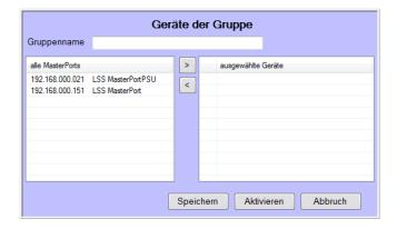
With the icon ("<") you can deselect unused devices from the group. Green point in front of the entries means these devices are accessible and can be programmed.
