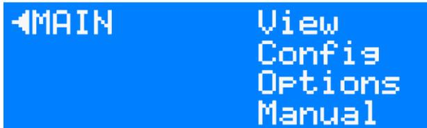
In the initial state, the device displays one of the 11 information pages. Pressing the encoder wheel for 1 second takes you to the main menu of the LSS PowerDim. The menu structure is hierarchical and includes submenus for information, function settings and general device settings. This results in level 1 (right-hand column) being labelled View, “Config” and Options. The structure of the submenus is described below.
