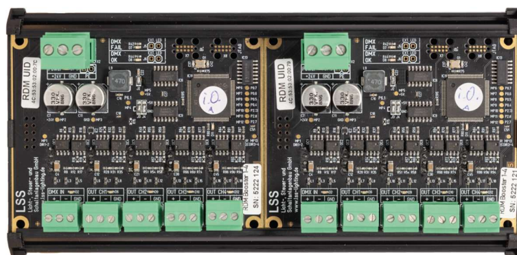
Example of a double booster with two LSS DMX Boosters 1 in 4
